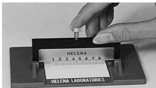
Fig. Applicator system used with the *Zip Zone* electrophoresis chamber. *Courtesy of Helena BioSciences.*
