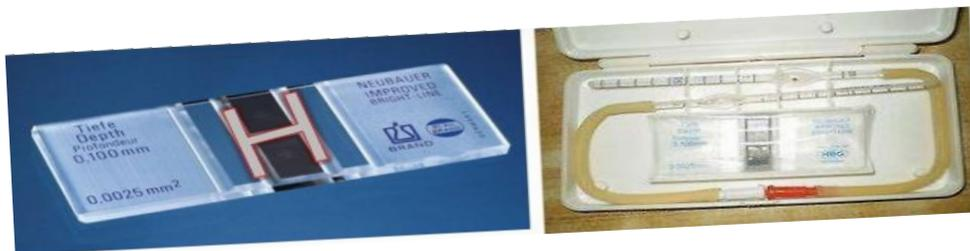
A thick glass slide with H shaped moats in it. The area between two lines of H (center) is 0.1 mm in depth. Moat prevents mixing of 2 samples on either side of chamber.
