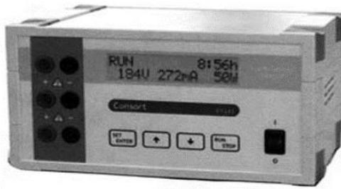
Fig. EV 243 Power Supply suitable for cellulose acetate hemoglobin electrophoresis with integral digital timer.
